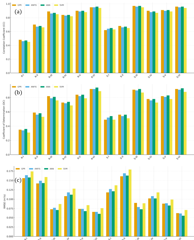
Fig. 6 Results for scenarios of the best models under rough-bed and smooth-bed conditions: (a) CC, (b) DC, and (c) RMSE
